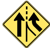
Added Lane (from right, no merging required)
